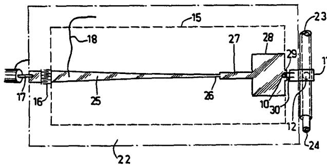
As a result the terminal impedance, which has been transformed very frequency-selective to a very high value in situ of the second coupling hole, is transformed to a very low value at the first coupling hole and very little power is dissipated in this low impedance, so that a considerable improvement of the circuit efficiency has been achieved.
